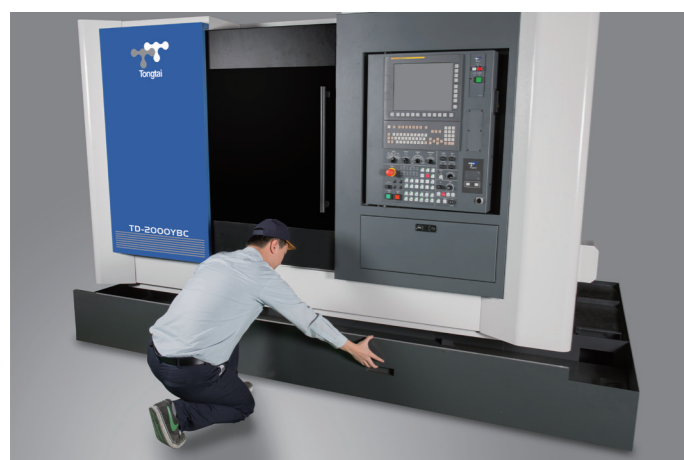
Coolant tank is able to be pulled from the front of the machine. It saves floor space and facilitates the maintenance.
