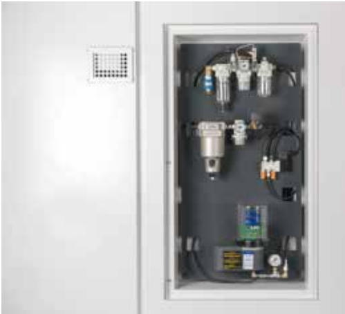
Through centralized management of pneumatic solenoid and lubrication pump, it made the daily maintenance easy.
