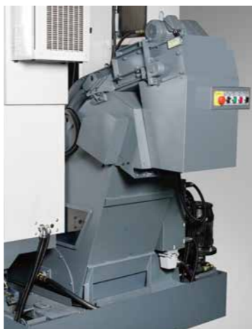
Coolant tank capacity: 700 L(80% full)
