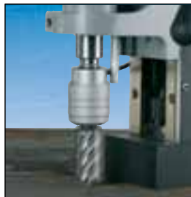
Drilling with core drills
