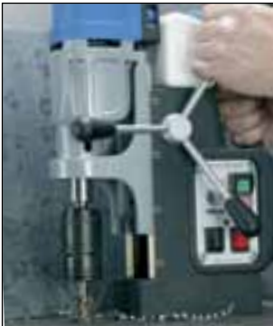
Tapping quick-change chuck size 2 for taps M8 – M16
