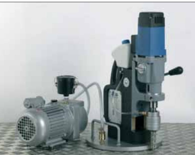
Vacuum plate for channelled plates: ZAV 300
