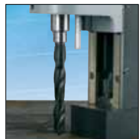
Drilling with twist drills
