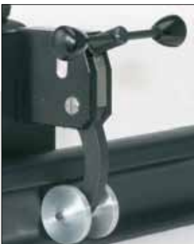
The quick-action clamping device exerts a pressure of 1.2 tons onto the rail foot, thus creating the required stability during drilling.
