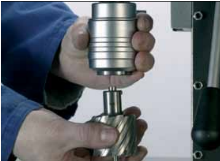
Quick tool change saves time and cost: Realized by the BDS Keyless quick-change drill system.
