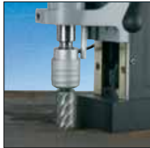
Drilling with core drills
